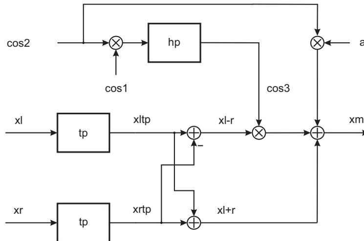
where  $h_{TP}$  is an ideal low-pass filter and  $h_{HP}$  is an ideal high-pass filter. The cutoff frequencies of the filters are identical at  $\Omega_C$  and the following applies:  $\Omega_C < \Omega_P$ .
